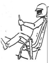
The shoulder harness should be mounted behind the driver and above a line drawn downward from the shoulder point at an angle of 40 degrees with the horizontal.
